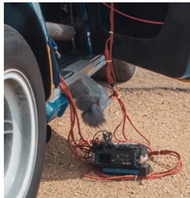
/ Zoom F8n and cables, with well-protected exhaust mics mounted on door sill
